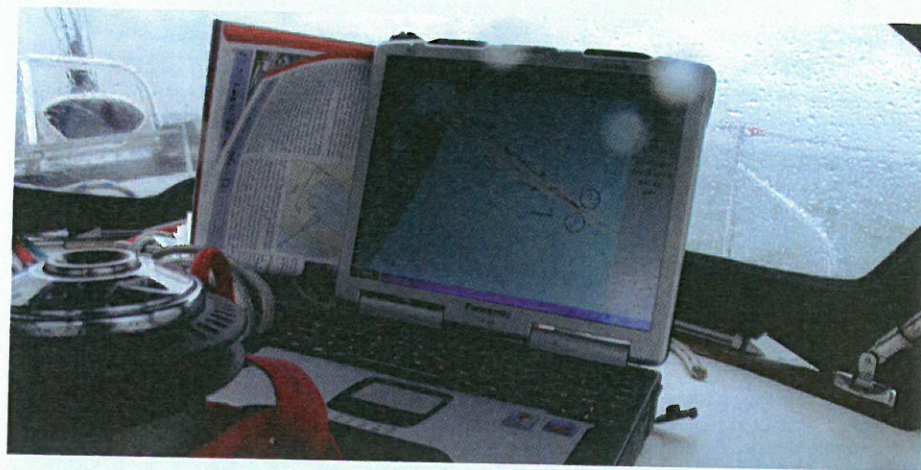
▲ The Panasonic Toughbook with internal GPS and charts is a handy back-up plotter.
