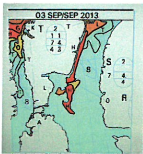
▲ Sea ice symbols are in the shape of eggs, and concentrations are graded 0 to 10/10ths, where 0 is open water and 10/10ths is uniform solid ice. A sailing yacht should in general not venture into conditions above 3–4/10ths ice.
